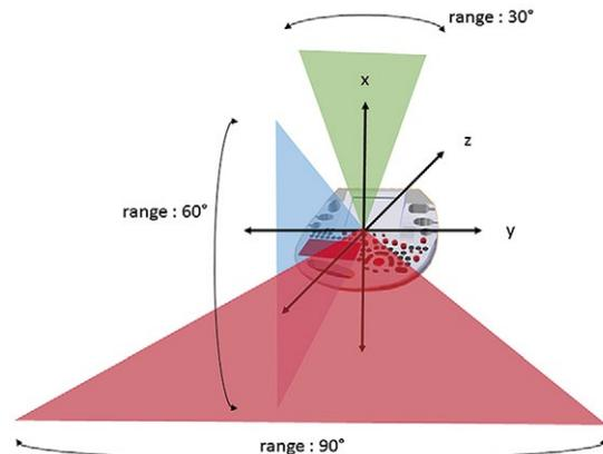
**Fig 3.** Illustration of the possible recognition planes, angles and dimensions of the modelled CAD console
